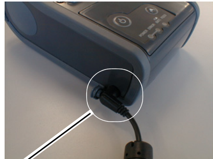
Connect the external power supply here after opening the cap
